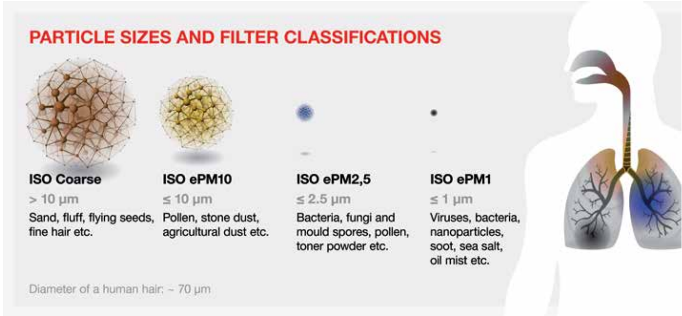
Particle sizes and filter classification according to the new ISO 16890 air filter standard
