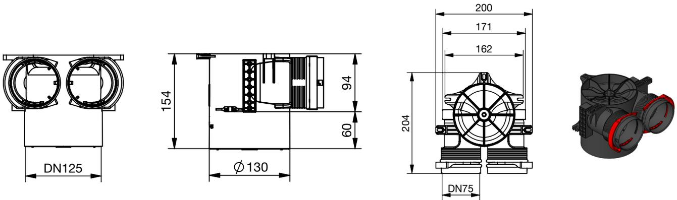
ComfoCase TVA housing, 2xDN90, DN125, lateral, H=410
