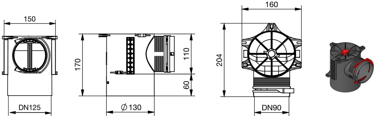
*ComfoCase TVA housing, 1xDN90, DN125, lateral, H=410, including adjustable mounting brackets*
