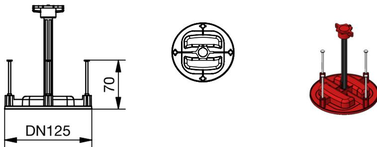
*ComfoCase mounting bracket set for TVA, 10 pieces, including screws*
