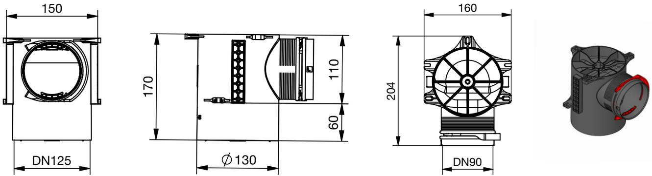
ComfoCase TVA housing, 1xDN90, DN125, lateral, H=410
