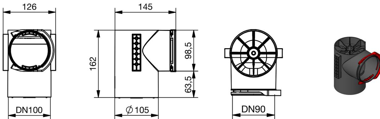
ComfoCase TVA housing, 1xDN90, DN125, straight, H=163
