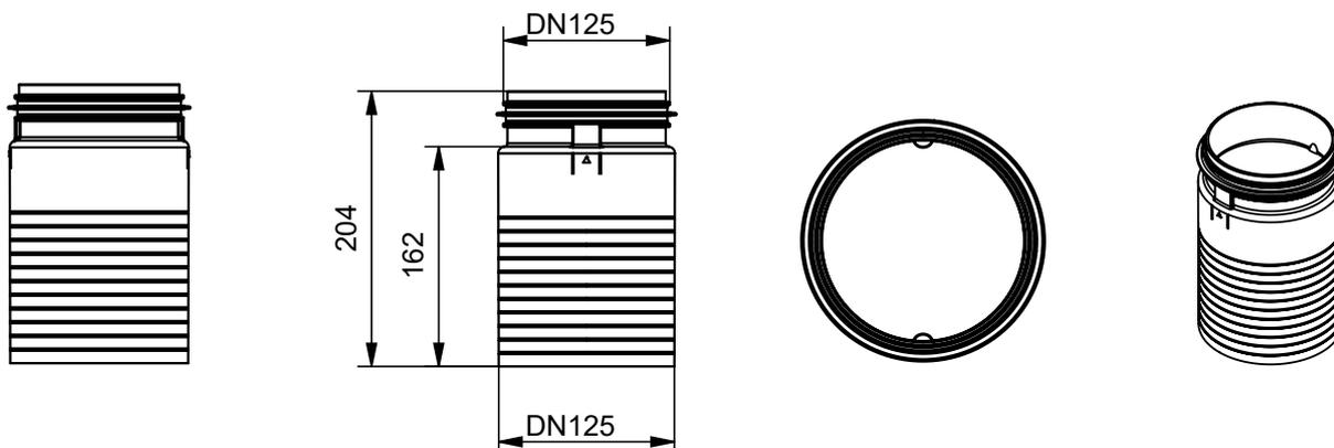
*ComfoCase fixing kit for TVA, DN125, for concrete installation, including nails*
