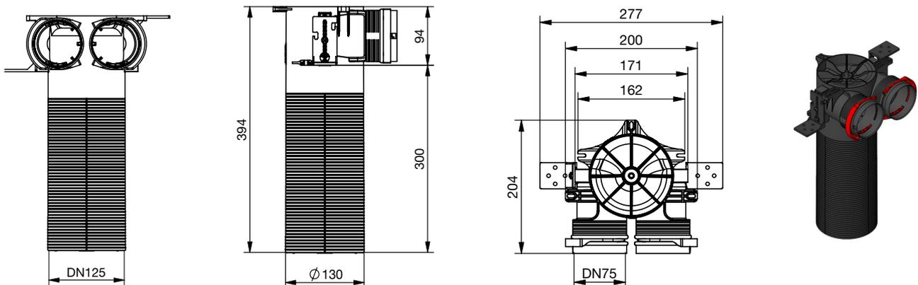
ComfoCase TVA housing, 2xDN75, DN125, lateral, H=394
