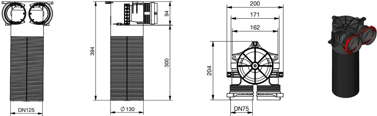
ComfoCase TVA housing, 2xDN75, DN125, lateral, H=154
