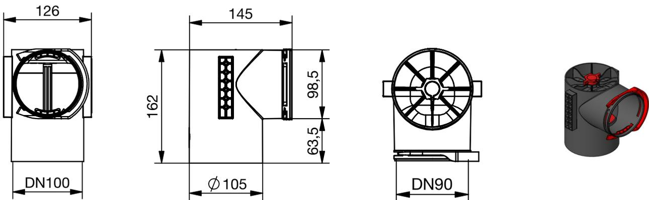
ComfoCase TVA housing, 1xDN90, DN100, lateral, H=162
