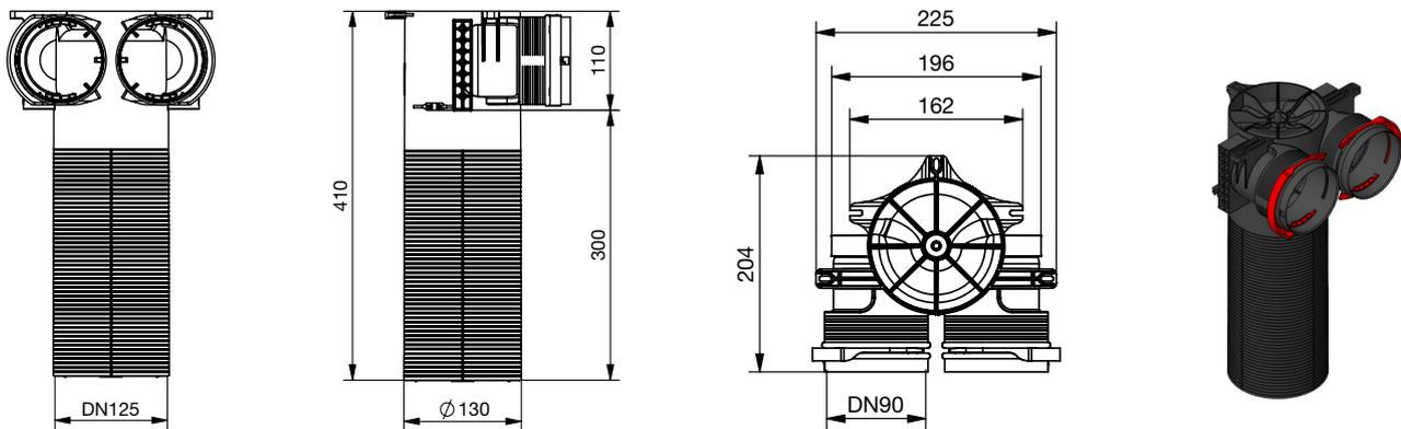
ComfoCase TVA housing, 1xDN90, DN125, lateral, H=170
