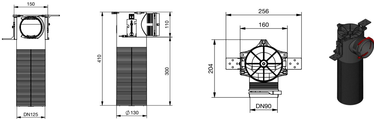
*ComfoCase TVA housing, 2xDN75, DN125, lateral, H=394, including adjustable mounting brackets*
