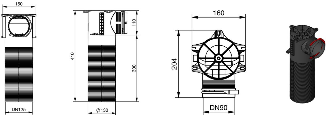
ComfoCase TVA housing, 1xDN90, DN100, lateral, H=162, including fixing kit for concrete formwork
