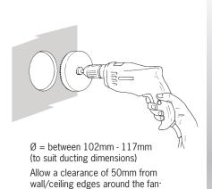
Cut the duct to depth of the plasterboard or tiled wall with slight fall to exterior (Make provisions for cable).
