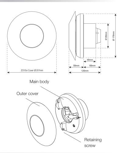
The unit can be installed on a wall, window (with separate adaptor kit) or ceiling mounted and ducted.
