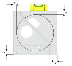
Fix the bottom cover in place in the four fixing points on the façade.
