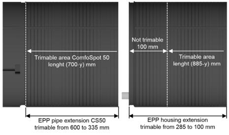
Trim using a suitable tool (utility knife) around the circumference and at a right angle to the axis of symmetry of the molded EPP parts.
