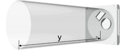
If the dimension y is > 700 to 885 mm, then only the EPP housing extension (1) needs to be trimmed by (885-y) mm. If the dimension y is 600 to  $\leq$  700 mm, both the EPP housing extension (1) and the EPP pipe extension for the ComfoSpot 50 need to be trimmed by 185 mm and (700-y) mm respectively.
