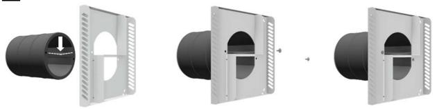
With the bottom cover installed, push the EPP housing extension into the PVC wall mounting pipe and use suitable fixing materials to fix the bottom cover to the four fixing points (shown as long holes) in a horizontal position on the façade.
