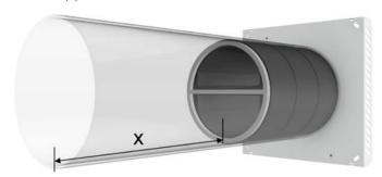
In the EPP pipe extension area, trim the **ComfoAir 70** by (600-x) mm.
