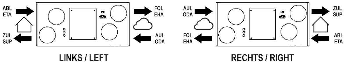
Fig. 19: Arrangement of the air connections Unit version LEFT and unit version RIGHT
