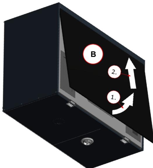
Fig. 28: Opening the front panel
