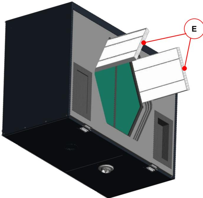
Fig. 30: Pulling out the filters
