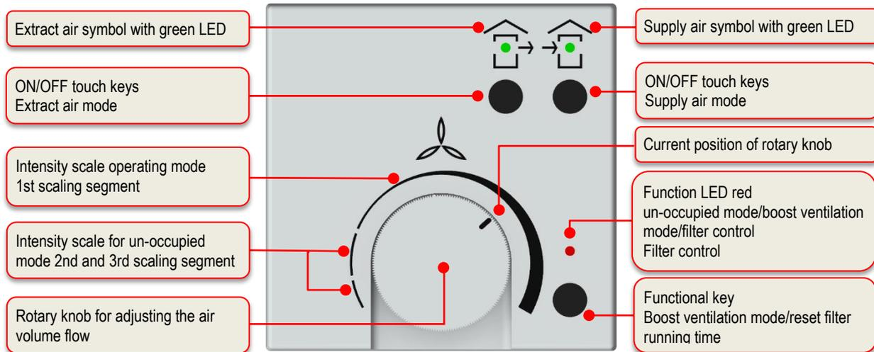
Fig. 2: Operation and information fields control panel
