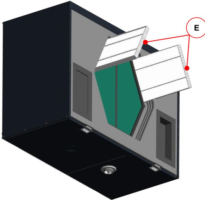
Fig. 6: Pulling out the filters
