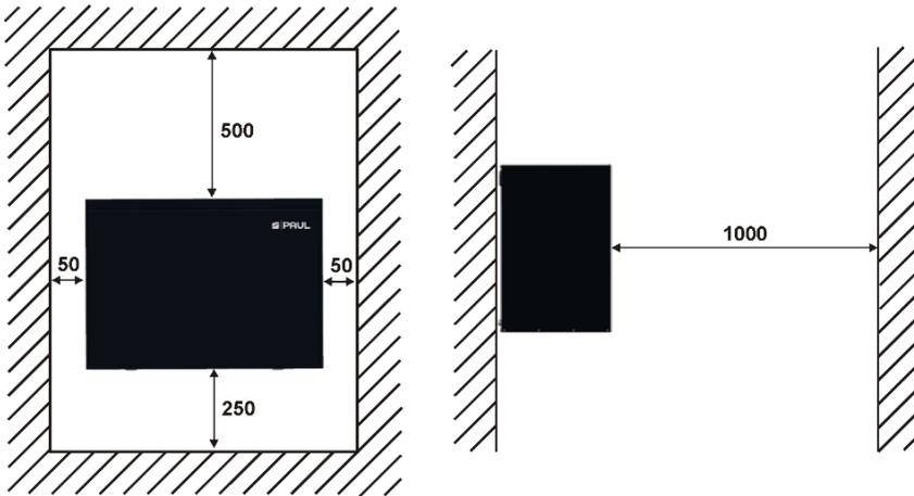
Fig. 8: Distances from adjacent surfaces in mm
