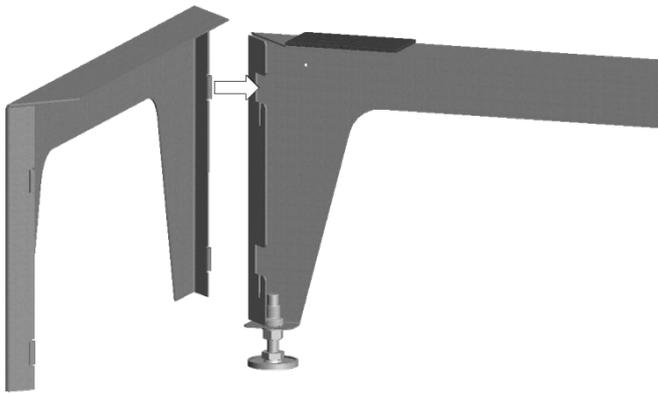
*Fig. 14: Assembling the base parts*
