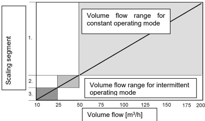
Fig. 26: Diagram 2, assignment of volume flow ranges
