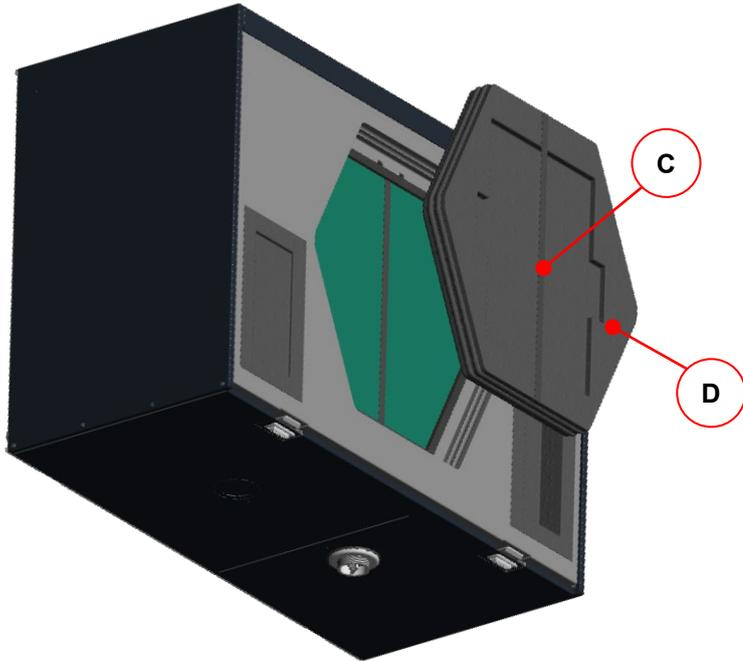
Fig. 29: Pulling out the EPP foam cover
