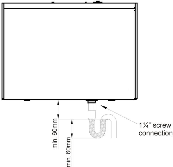
Fig. 22: Condensate drain (version LEFT)
