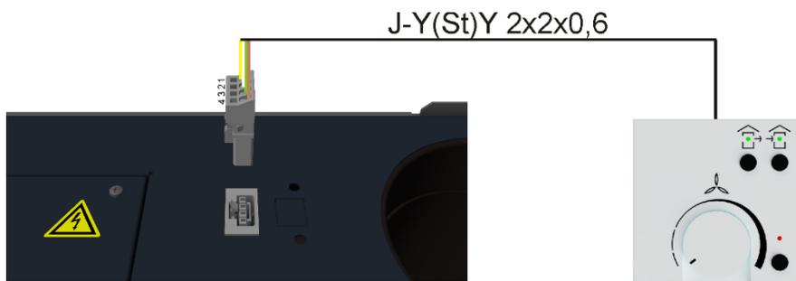
Fig. 24: Connecting cable with flat connector plug
