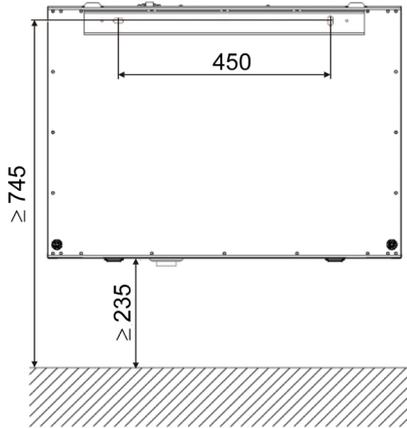
Fig. 10: FFL distance for wall mounting (version LEFT)
