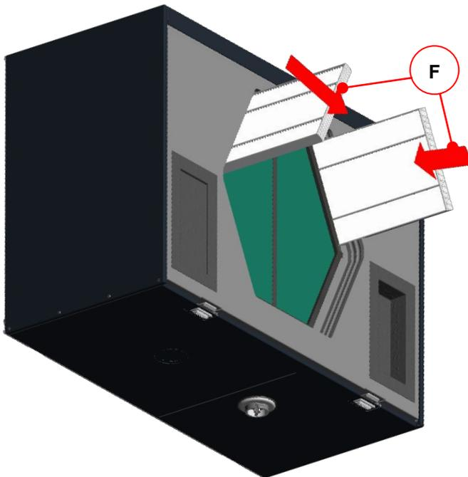
Fig. 7: Inserting the new filters according to the direction of flow
