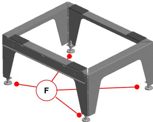
Fig. 18: Aligning the floor stand
